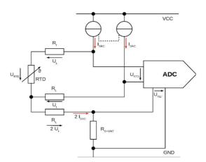
The 16-bit AD converter used directly measures the ratio between the voltage at the sensor and the supply current, i.e. the actual resistance value. A switchable gain factor allows optimized adaptation to Pt100 or Pt1000 sensors.
