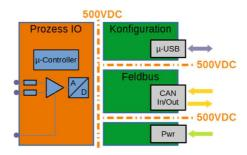
In the RAIL version, the CAN bus is routed in the same cable as the power supply. Here, the ground potential of the power supply is identical to that of the CAN bus. The isolation to the process IO is designed for 1.7 kV DC.
